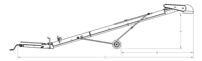
A = Discharge Height B = Wheel Clearance C = Overall Length
