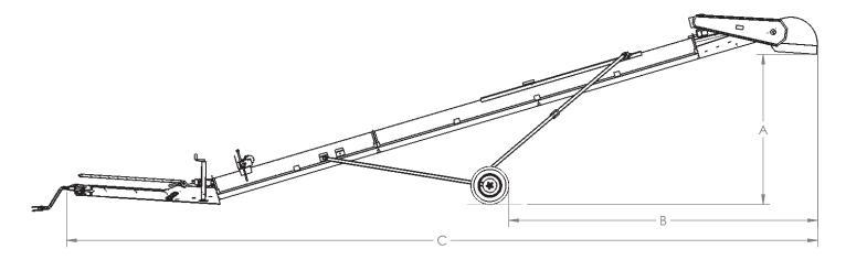
A = Discharge Height B = Wheel Clearance
