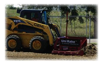
The UniRake<sup>™</sup> is a dirt rake that features replaceable teeth with two choices in length, and comes with an optional blade which is operated by a hydraulic lift with flow control.
